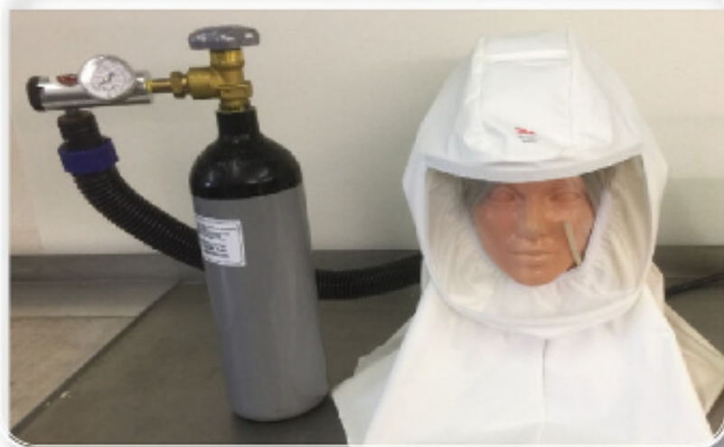
3M Versaflo headgear connected to a cylinder of compressed gas
