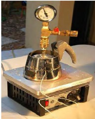
Fig 20.2 (above): The 'Single Shot' Autoclave
