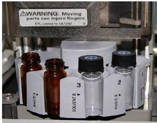
Fig 20.6: Vials of barbiturate solution for assay using gas chromatography
