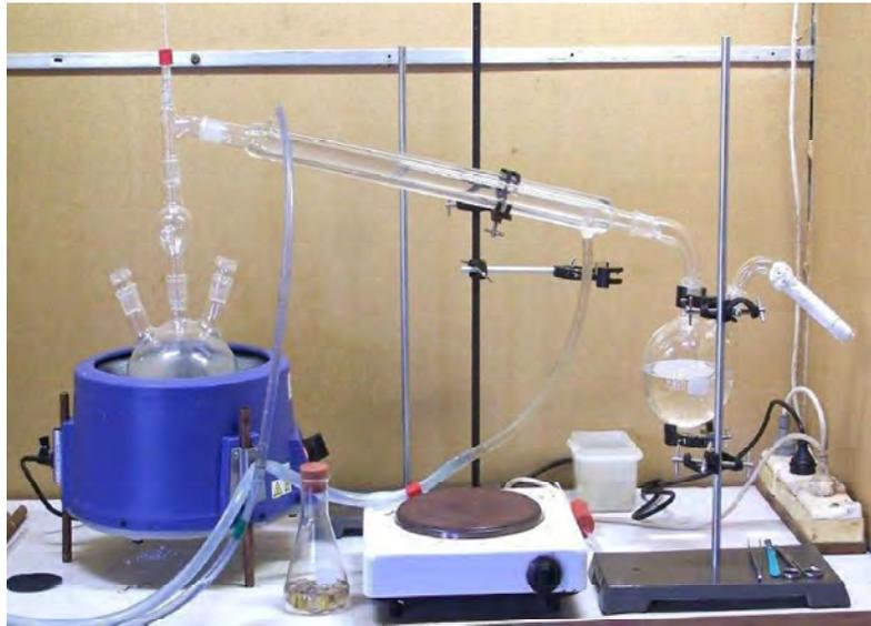
Fig 20.5: Glass distillation system
