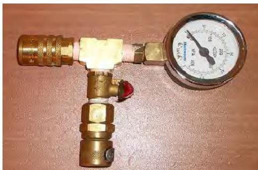
Fig 20.4: Autoclave pressure head
